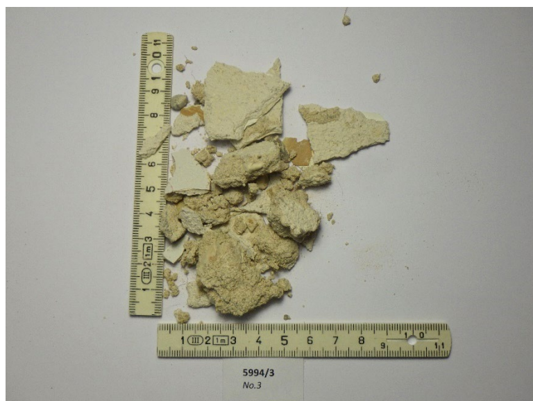
Figs 5 to 6: Sample 5994/3: Photographs of plaster sample received for test (dry condition).
