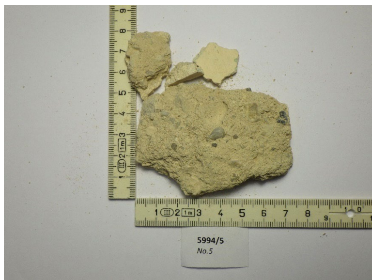
Figs 9 to 10: Sample 5994/5: Photographs of plaster sample received for test (dry condition).
