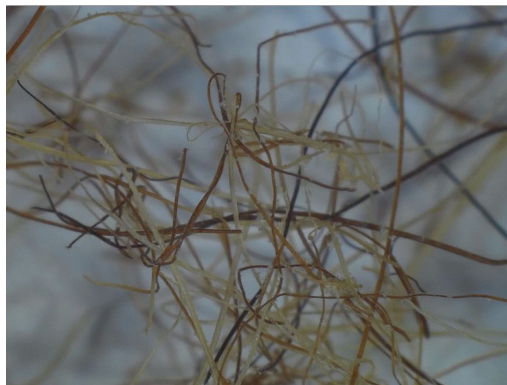
Figs 18 to 20: Plaster basecoat sample 5994/3.3 – Showing respectively: • Extracted insoluble sand and aggregate component (dry condition) • Silt and clay / fines component (dry condition, magnified) • Hair reinforcement (magnified)
