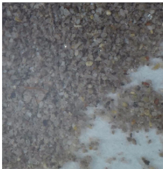
Figs 16 to 17: Plaster topcoat sample 5994/3.2 – Showing respectively: • Extracted insoluble sand and aggregate component (dry condition) • Silt and clay / fines component (dry condition, magnified)
