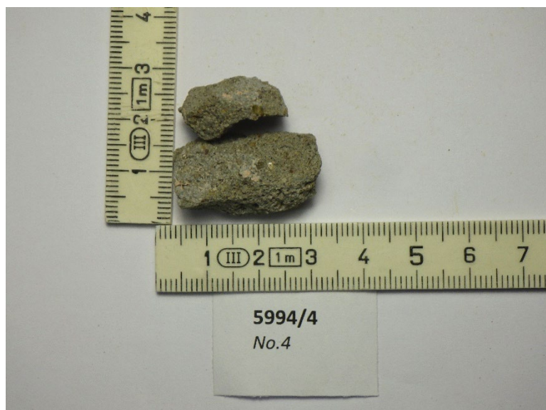
Figs 7 to 8: Sample 5994/4: Photographs of plaster sample received for test (dry condition).
