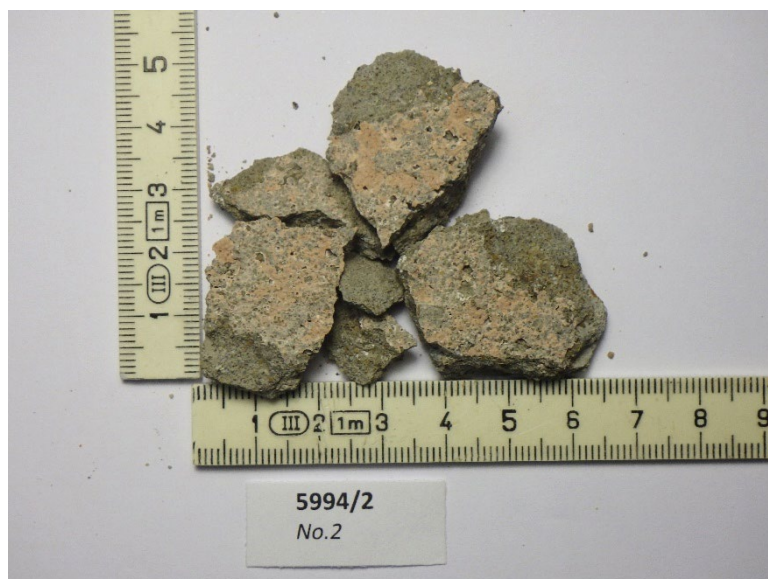
Figs 3 to 4: Sample 5994/2: Photographs of plaster sample received for test (dry condition).
