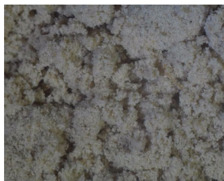
Figs 18 to 20: Plaster basecoat sample 5994/3.3 – Showing respectively: • Extracted insoluble sand and aggregate component (dry condition) • Silt and clay / fines component (dry condition, magnified) • Hair reinforcement (magnified)
