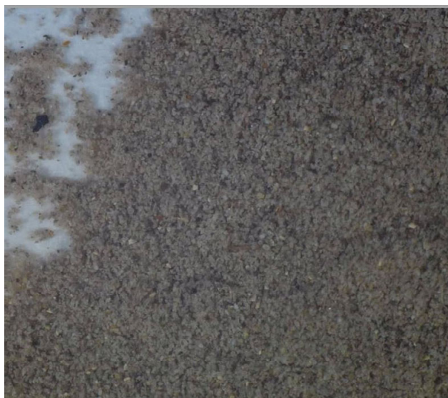
Figs 23 to 24: Plaster topcoat sample 5994/5.2 – Showing respectively: • Extracted insoluble sand and aggregate component (dry condition) • Silt and clay / fines component (dry condition, magnified)
